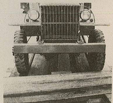
Fig. 6 - The rails won't tear the wheels off your trucks if you pave 'em with lumber.
