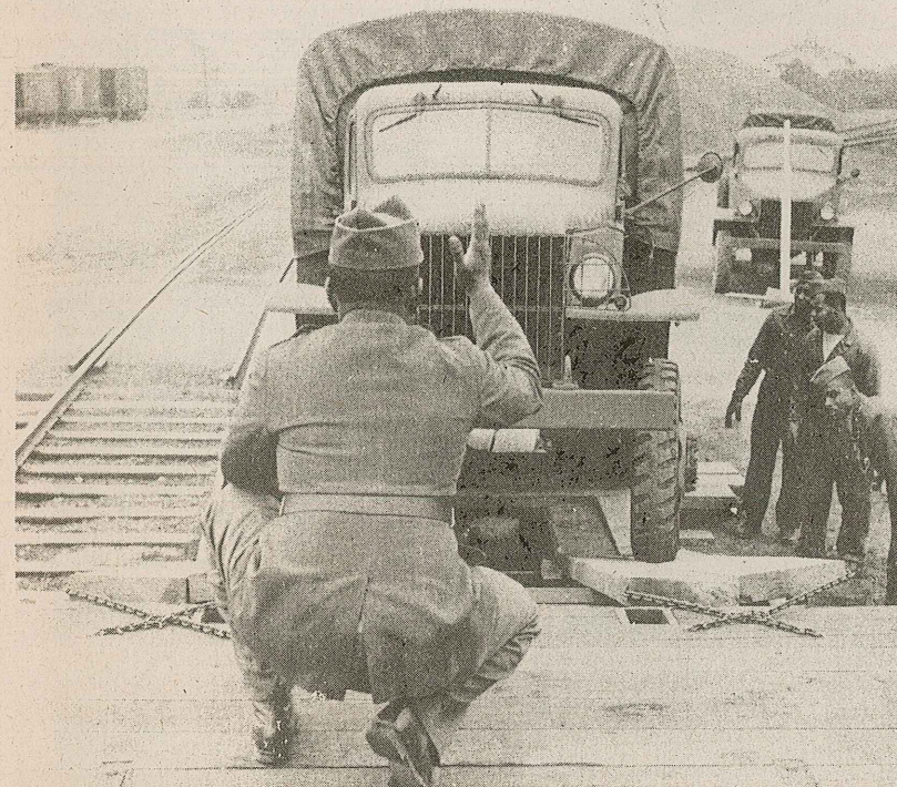
Fig. 7 - Man guides truck. The truck-guider is the driver's eyes. Sees all, tells all. Any heckling or added directions from the nickel seats will drive the driver crazy.
