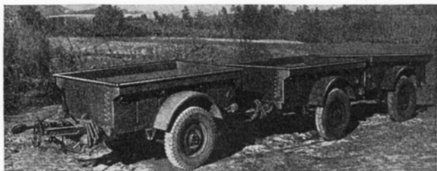
Figure 3.—Three \frac{1}{4} -ton trailers lashed in series.
