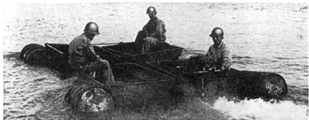
Figure 7.—Four-trailer raft with 55-gallon drums as auxiliary flotation.
