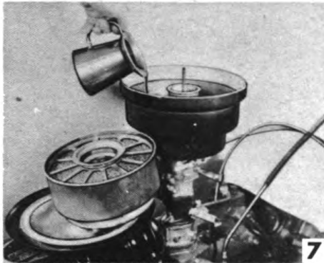
7 CARBURETER AIR CLEANER (Clamp Mounted Type)—OE Remove cover and element. Check oil level and cleanliness. Clean in dry-cleaning solvent. Dry thoroughly. Install reservoir and fill to "oil level" mark with OE, SAE 50 above +32 F or SAE 30 between -32 F and 0 F. From 0 F to -40 F use SA. Below -40 F operate dry. Install dry element and cover.
