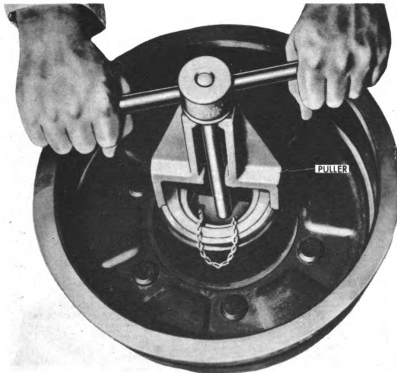
Figure 200—Removing Inner Cone and Rollers (Puller 41-P-2898)
