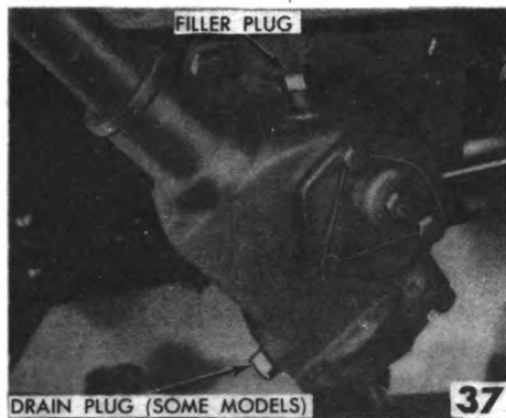
STEERING GEAR HOUSING—GO Filler plug. Drain plug on late models. Pump gun. Remove drain plug (when used) to drain housing. Reinstall plug and fill to level of filler plug hole.
