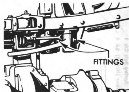
2 FITTINGS (1 EACH PEDAL). PRESSURE GUN. LUBRICATE FROM UNDER VEHICLE.
