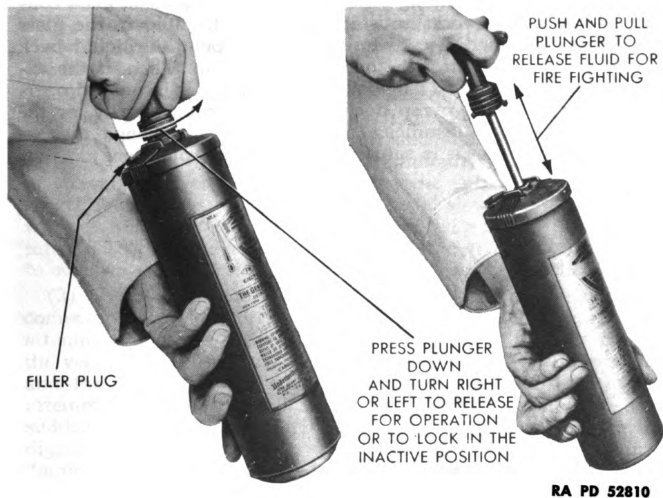
Figure 31—Operating Fire Extinguisher
