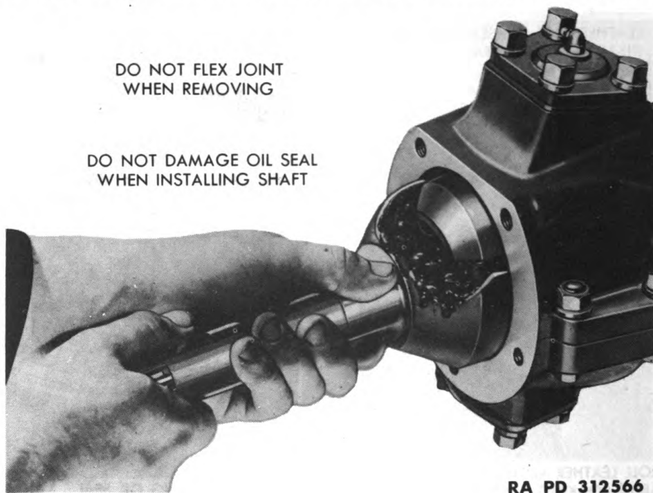
Figure 157—Removing Universal Drive Assembly
