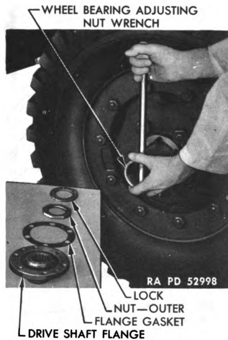
Figure 153—Adjusting Front Wheel Bearing
