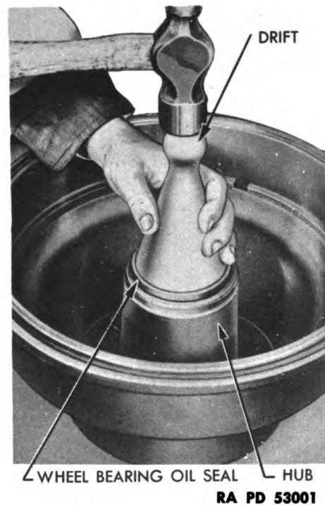
Figure 156—Installing Wheel Bearing Oil Seal with Drift 41-D-1535-50
