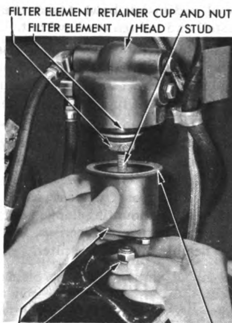
FILTER ELEMENT RETAINER CUP AND NUT FILTER ELEMENT HEAD STUD BOWL STUD NUT AND GASKET BOWL BOWL GASKET
