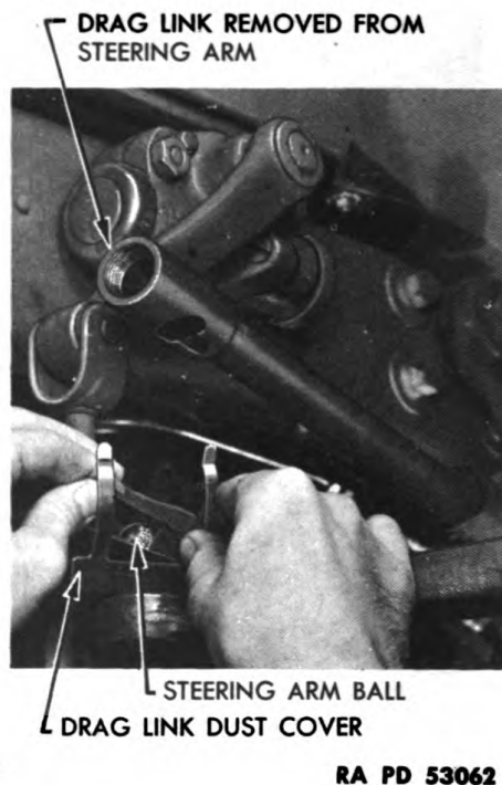
Figure 191—Removing Drag Link from Steering Arm
