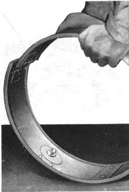
COLLAPSING TIRE BEAD LOCK RING
