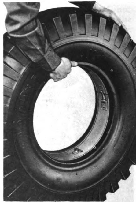
TIRE BEAD LOCK RING INSTALLED
