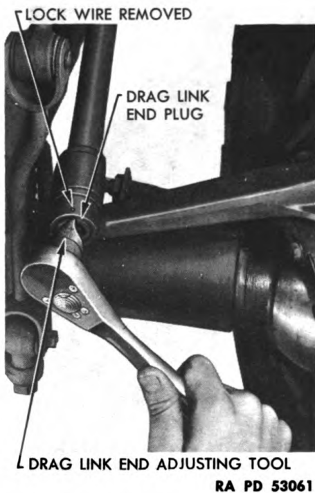
Figure 190—Adjusting Drag Link End
