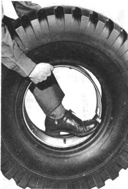
EXPANDING TIRE BEAD LOCK RING IN TIRE
