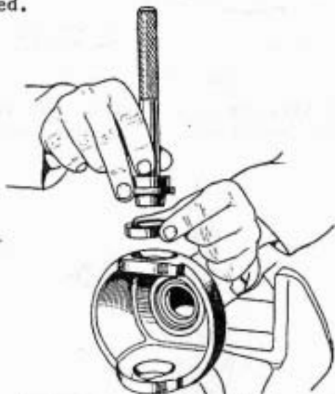
Replacing pivot bearing cups. Fig. 70
