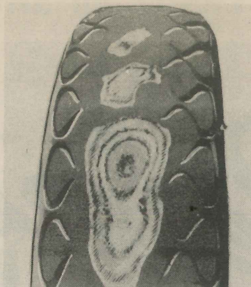
A GRABBY BRAKE is responsible for this condition - it's too late for anything.
