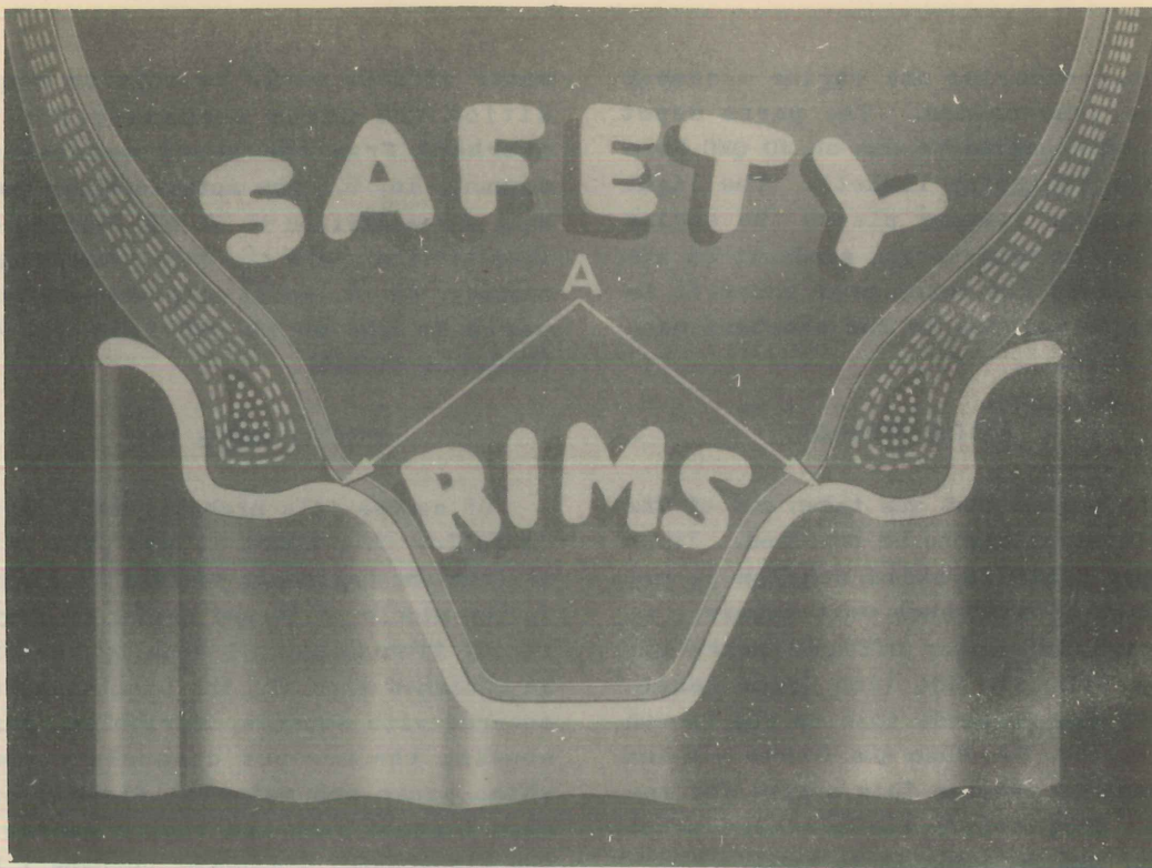
Figure 1 Cross section of tire and rim
